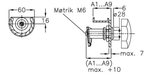
Door + frame thickness = 42-50Measure type = A6
